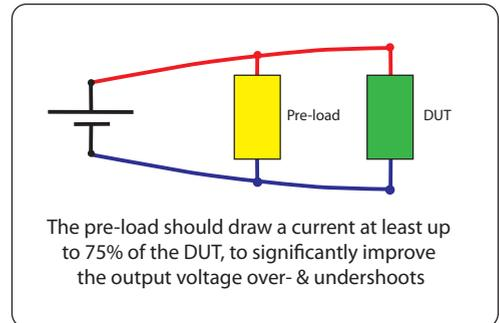
A disadvantage of using a pre-load is that twice as much DC output current is required. Fortunately, if you use AMETEK switching power supplies, additional power is relatively inexpensive. This makes using pre-load a much cheaper and more practical approach than specialized power supply sub-systems for this specific application.
