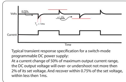
A typical application example where transient response is important is mobile phone testing. In this application, the DC power supply simulates the mobile phone's internal battery. When it begins to transmit, the current rise is very quick.
